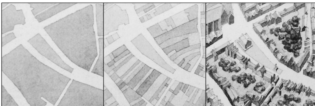
Figure 2.5 town plan, land use pattern, building fabric (left to right) (Source: Kostof, S. (1999), The City Shaped.)
