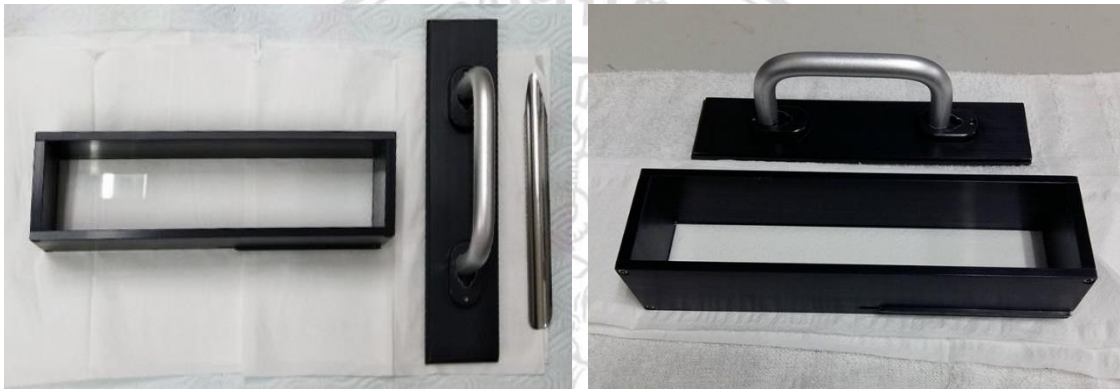
Figure 3.1 Coarse sample cell (width \times length \times depth, 5.7 \times 29.4 \times 2.0 cm)
