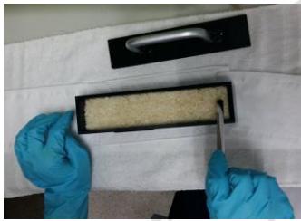
(D) Equalize the surface of sample by a spatula
