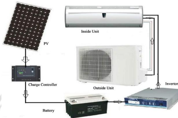
Figure 1.2 Solar air conditioning system [6].
