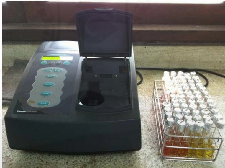
Figure 2-7 Spectrophotometer for analyzing the absorbance of sample
